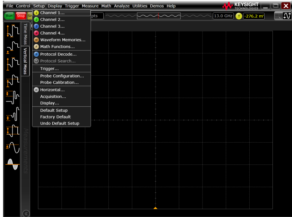
Figure 11 Channel Setup Window
